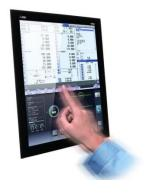
Mitsubishi Electric's M800W series is a 19-inch touch-screen vertical display on CNC control units; screen keyboard and document viewer accommodate multiple windows which can be customized by machine manufacturer vendors. While CNC screen is displayed on the upper half, the virtual keyboard, operator panel, document viewer or memo pad can be opened at the bottom. M800W series
