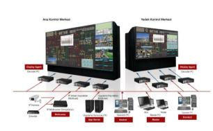
Thanks to S-SF architecture, control room videowalls no longer need a special videowall processor. Thanks to multiple redundencies incorporated in distributed network architecture without the need of an addition, fault tolerance is applied. In the case of a fault in a component, the role of that component will be assigned to another
