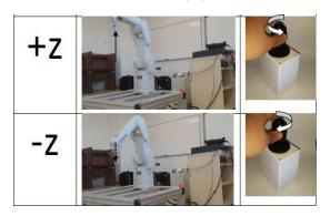
Another project performed with Mitsubishi Electric robot aims to control the robot arm by means of a 3D joystick connected from outside. Industrial robots, which are involved in a wide variety of tasks in manufacturing systems, are controlled with the help of keys on the teach pendant, and
